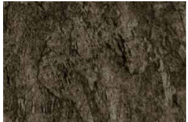
Luvata's CuCrZr fine grain structure
