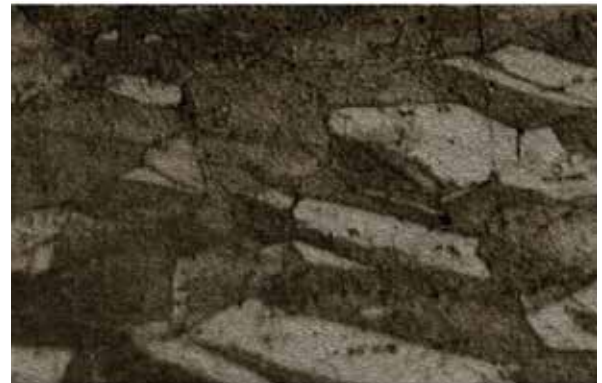
Conventional CuCrZr grain structure
