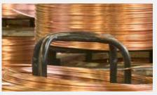
**Plating:** Luvata typically provides battery nail wire to the market 'pre-plated'. Plating is typically in the range of 0.5-2.0 microns of Bright Tin. Bare wire (to be post plated by the customer after nail forming) is also available.
