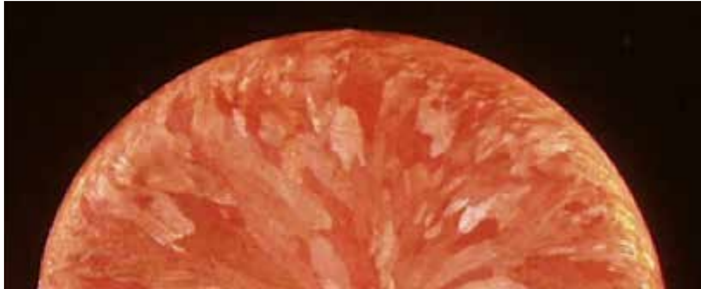
Figure 1. Luvata's anode balls contain large cast grains.
