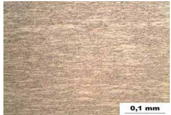
Grain structure of DSC with aluminum oxide
