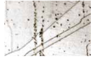
CuCrZr before and after annealing at 900°
