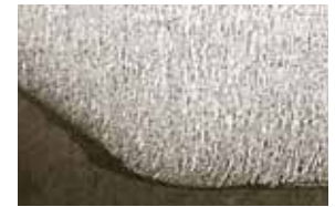
Nitrode after 1200 welds
